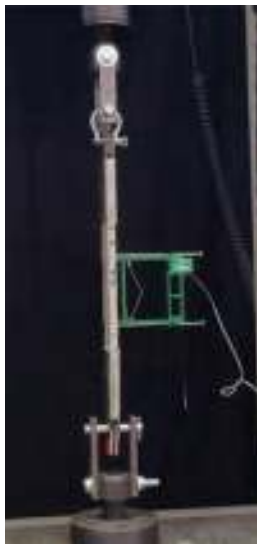
Fig. 3.2.1c—Tensile test with clevis-type grips.
